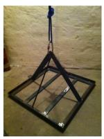
Substitute to wall/floor rigging's are Agit-Cirk's own metallic structure's. In this case the venue should provide 1000kg weights for the structures. This can be anything fitted to 60cm x 60cm structure (bags of sand, concrete tile 30x30cm etc.) We also need a black fabric to hide the weights.
